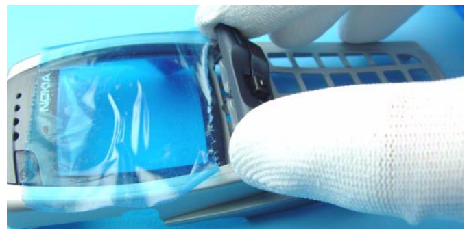
Remove Function Keys if needed. Use always new keys in reassembly!
