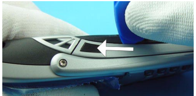
Place the SRT-6 between B-Cover and A-Cover and shift it carefully as shown in the picture. Note the correct position of the SRT-6, the tip should not touch the PWB.
