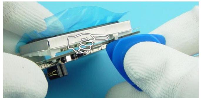
Release the snap on the other side of the engine and take away the LCD Module.
