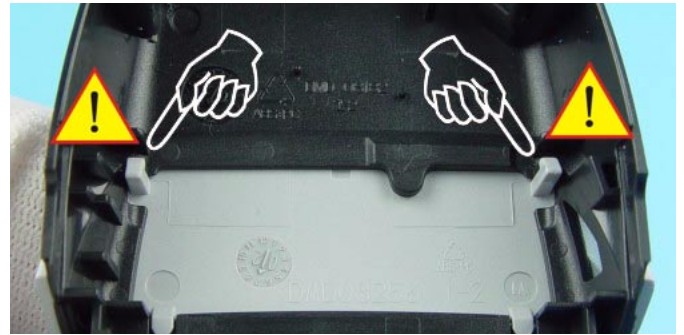
The Logo Bracket is attached with snaps to the B-Cover. Take care not to break the snaps when releasing the Bracket.
