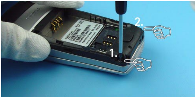
Unscrew the two TORX PLUS® size 6 screws using the order shown. For assembly, the reverse order and a torque of 17Ncm have to be used.
